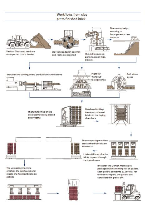
The flow diagram conforms with the requirements in the modular approach and shows the production phase A3 for brick production (Petersminde Teglværk only uses "soft stone press", no "extruder" and no "handcut"). The remaining phases are described below.
